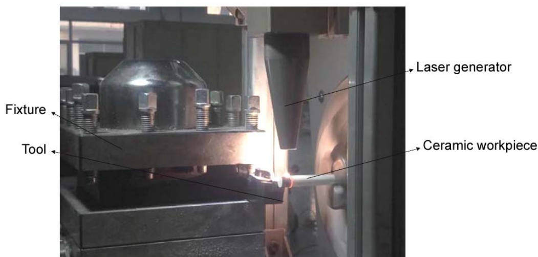
图 6 激光辅助机械加工 Figure 6 Laser assisted machining
